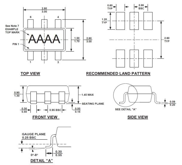
Figure 4. TSOT23-6/SOT23-6 Physical Dimensions
